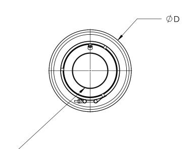
1NLET AND OUTLET DIAM ARE AVAILABLE IN 2.0", 2.25", 2.5", 2.75", 3.0", 3.5" AND 4.0" ID. OTHER SIZES IN IMPERIAL, METRIC, NPT PIPE AND ANSI FLANGES ARE AVAILABLE UPON REQUEST.
