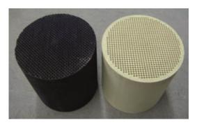
2) Silicon Carbide (SC) - Silicon Carbide substrate cores have a high thermal expansion rate with good mechanical strength. Silicon Carbide substrates have a higher melting point and a higher heat capacity in relation to Cordierite ceramic. Therefore a Silicon Carbide substrate core has a higher capacity per liter of filter volume in terms of PM mass in comparison to a Cordierite Ceramic substrate core. Silicon Carbide substrate
